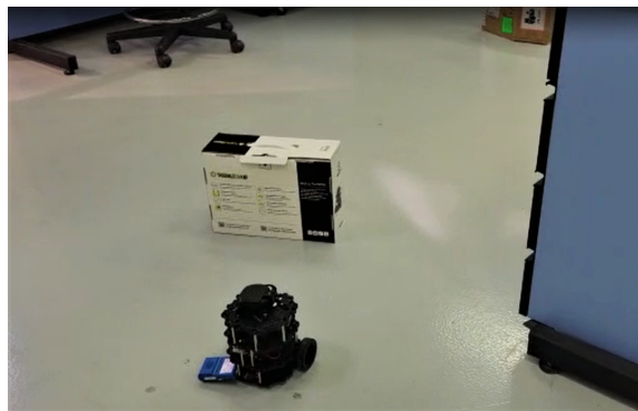
FIGURE 3.25: Autonomous navigation and obstacle avoidance using TurtleBot3 in the IoT Lab
