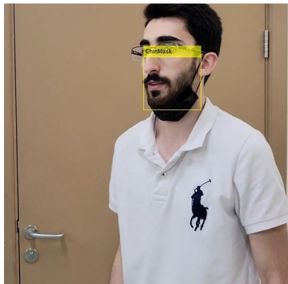
FIGURE 3.7: Mask under chin detection using YOLOv2 object detection
