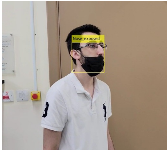
FIGURE 3.6: Nosed exposed detection using YOLOv2 object detection
