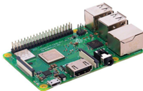
FIGURE 2.9: Raspberry pi 3B+ [11]
