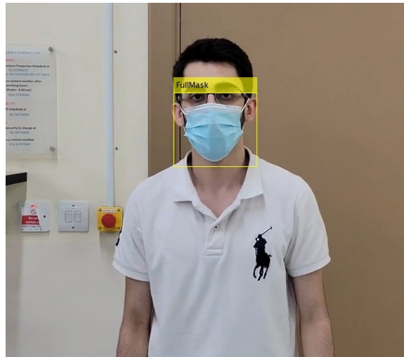
FIGURE 3.4: Full face mask detection using YOLOv2 object detection
