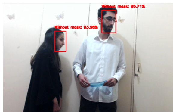
FIGURE 3.9: Face mask detection using tensorflow and openCV on two people without face masks
